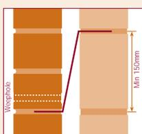
Horizontal DPC's should cover the full width of each leaf and not project into the cavity.
